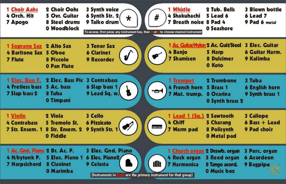
The ENSEMBLE key on the lower left puts 18 alternate instrument combinations at the touch of your finger. First press the ENSEMBLE key and then one of the instrument or number keys.
